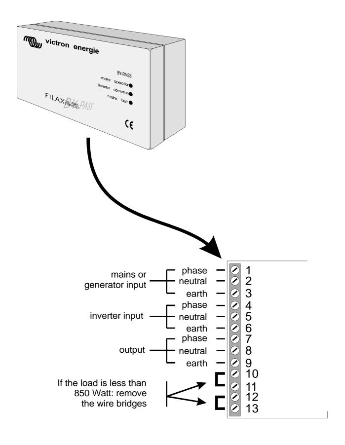
Figure 1. Connection diagram Filax
